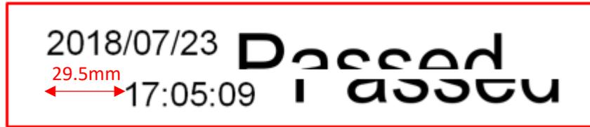
4. To set your offset first measure the distance between the start of printhead 1 and the start of head 2. Enter the results in millimeters (mm) into “print head offset” #2
