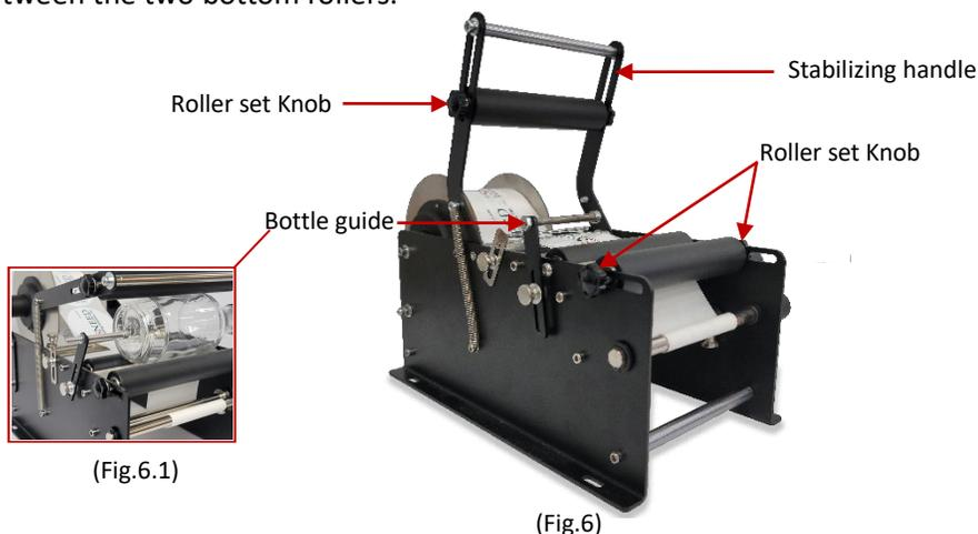
6. Utilize the bottle guide shown in Figure 6.1 to guarantee the bottle's stability and consistent positioning.
