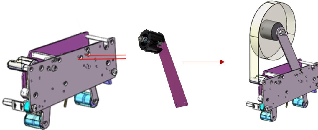
2. Next Install the tape onto the tape wheel so that when you pull the tape down the adhesive side is facing outward.
