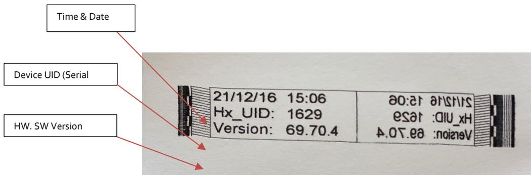
Figure 11. Print Test Result
