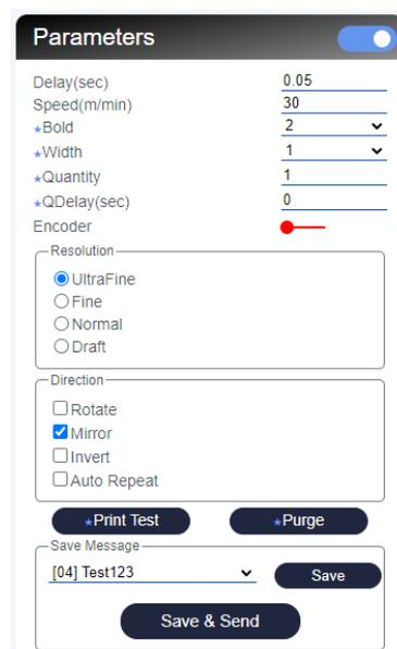
Figure 14. Print Parameters Advance Mode
